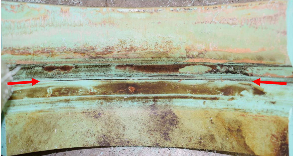
Figure 9. Sample E1 gasket race area with circumferential fracture after initial cutting and removal from the bell. Note circumferential fracture at the approximate mid-height of the image (at red arrows), as well as residue present in the gasket race “behind” where the gasket was previously placed. Non-pressure side of the gasket and bell lip are at image top, while the pressure side of the gasket and bell barrel are at image bottom.
