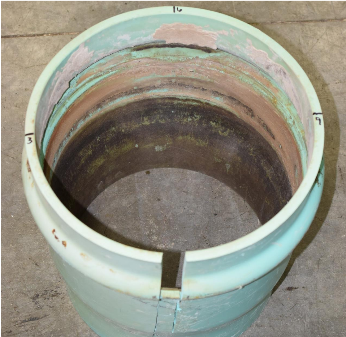
Figure 17. Sample E2 just after extraction of the spigot and gasket by sectioning and disassembly. Note fine grained debris present on both sides of the gasket race. Also note circumferential fracture at the gasket race at the as-installed 12 o'clock location (near image bottom with small section missing).
