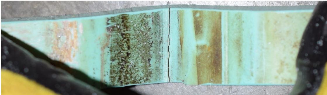
Figure 5. “Steps” present within the Sample E1 fracture. Inside diameter view, with circumferential fracture in the middle of the image running top to bottom. Each “step” represents a distinct fracture origin.
