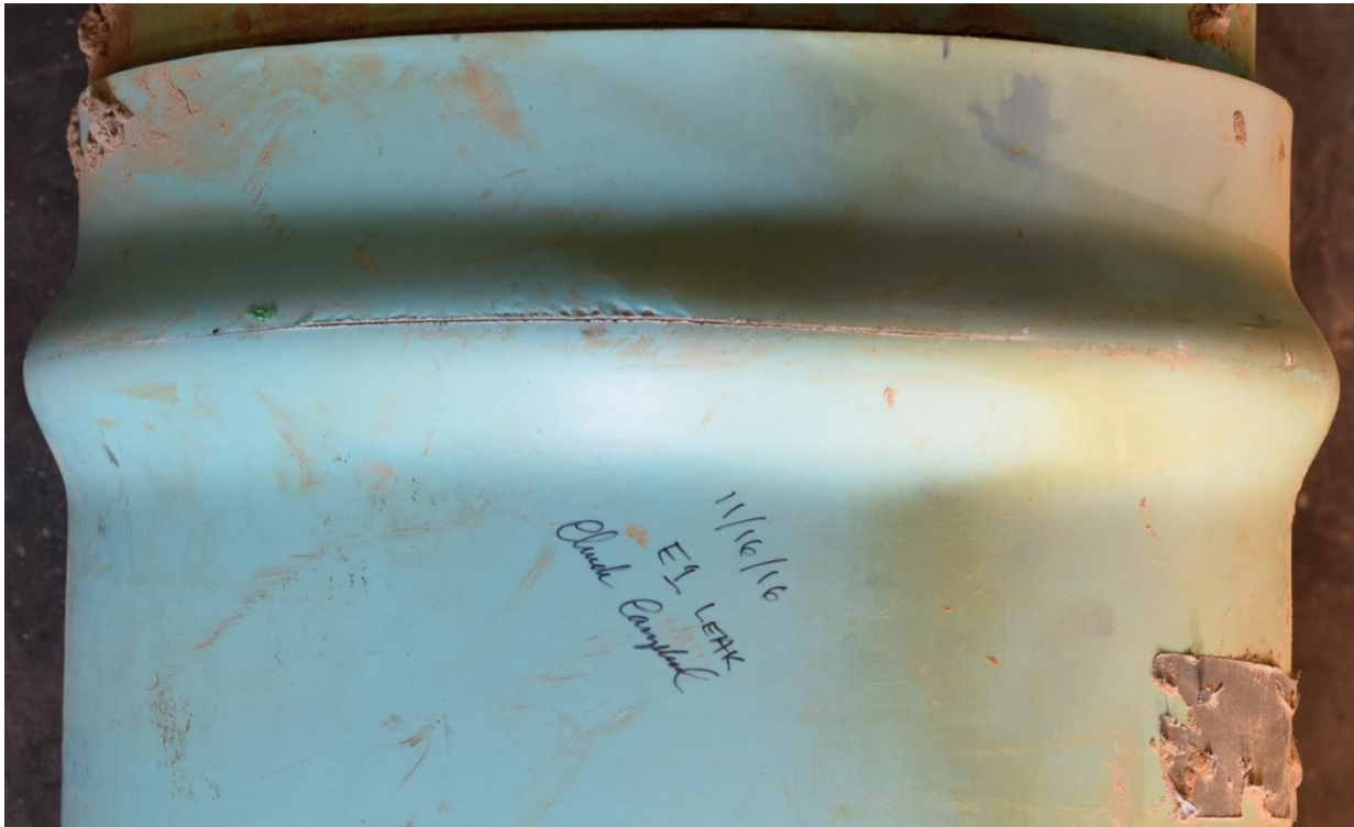
Figure 4. Digital image of Sample E1 with circumferential brittle fracture located at the “crown” of the gasket race. Note macroscopically brittle structure, with slight erosion near the center of the fracture.
